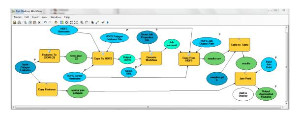
**Fig. 1.** The geoprocessing workflow running on ArcGIS to submit a MapReduce job of the spatial-join operation on Hadoop.
