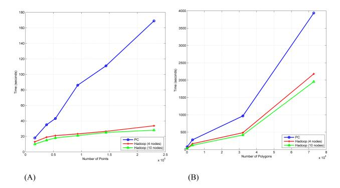
**Fig. 1.** The computation time curves of Hadoop-based spatial joins and a single desktop PC: (A) increasing the number of joined points; (B) increasing the number of target polygons.
